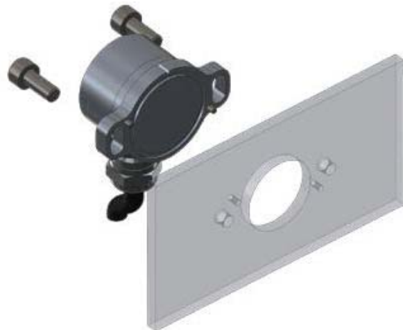
Mounting example of the variant for drilling pattern P: Mount using 2 M4 screws, exact alignment is ensured using cylindrical pins h8 1.5 pre-assembled at encoder (screws not included)
