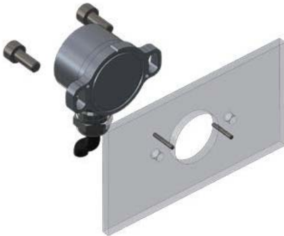
Mounting example of the variant for drilling pattern S Mount using 2 M4 screws, optional exact alignment using 2 cylindrical pins h8 1.5 (e.g. ISO 2338 B) (screws and pins not included)
